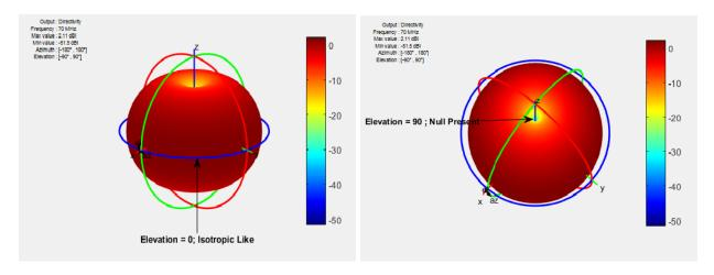
The dipole is omnidirectional around the E-plane, or elevation angle. The null is present in the H-plane, or azimuth angle.
